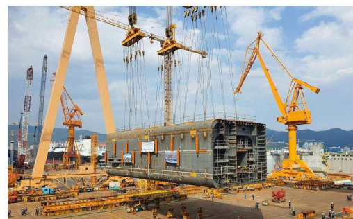
Keel laying and lift of the first gigablock onto the skidway in South Korea
